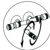
When installing, make sure that the hose is not kinked or compressed. Furthermore, make sure that the hose does not run too close to possible heat sources in the terrarium. This can lead to deformations or fire hazards. After connecting, align the spray nozzles in the desired directions. Take special care that no electrical devices (e.g. lamps, sockets) are sprayed. When using a nozzle for spraying, make sure that the nozzle of the main motor is firmly tightened clockwise.
